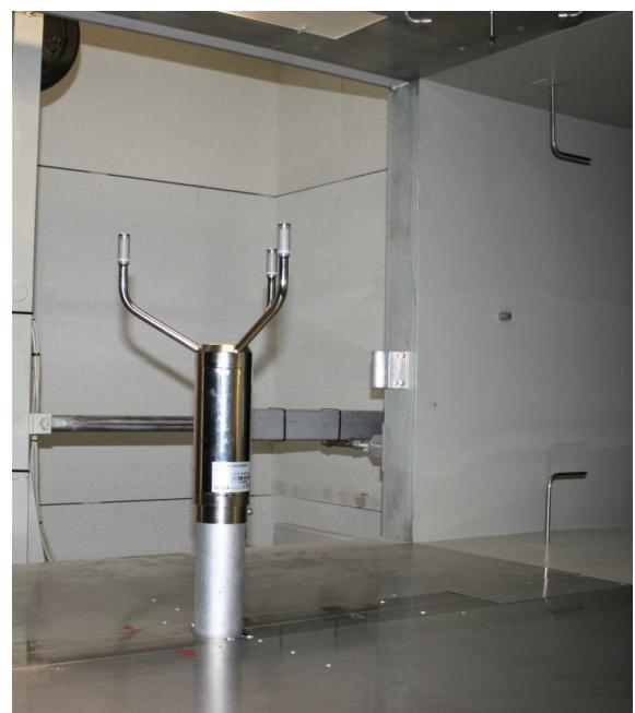
Calibration set-up of the anemometer calibration in the wind tunnel of Deutsche WindGuard, Varel. The anemometer shown may differ from the calibrated one. Remark: The proportion of the set-up are not true to scale due to imaging geometry.
